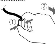
Hold the connector tightly (①), then pull it out (②).
